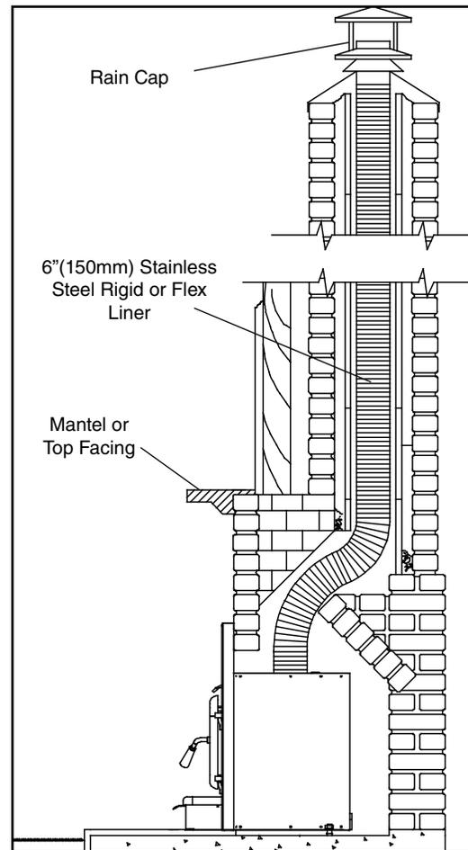
**Full Flue Liner:** where a listed stainless steel rigid or flexible liner extends from the Insert flue collar to the top of the chimney.
